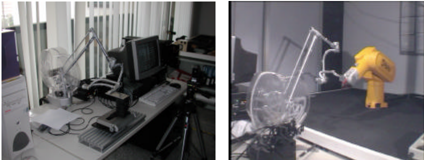
Fig. 1 Mechanical slide (left) and a Staubli Unimation RX60, having 6 DOF (right)
