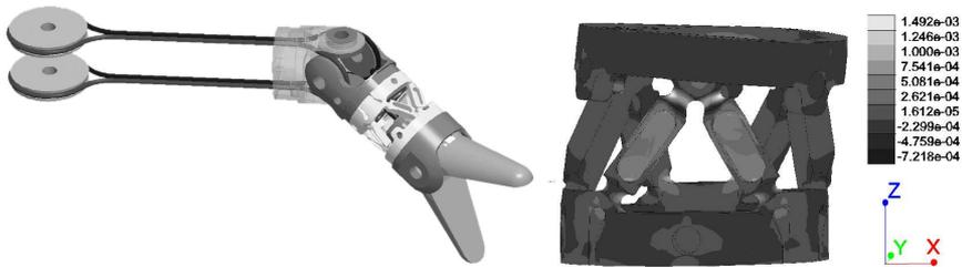
**Fig. 1.** Articulated joint with drive cables (left) and average  $xz$ -strain on force/torque sensor for load  $F_x = 20\text{ N}$  (right)
