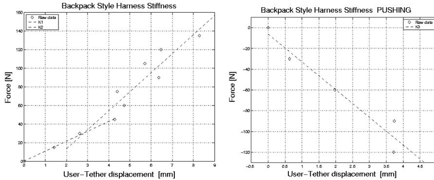
**Fig. 3.** *Left:* Bilinear interpolation for the estimate of a backpack-style harness stiffness in pulling action. *Right:* behavior in pushing.
