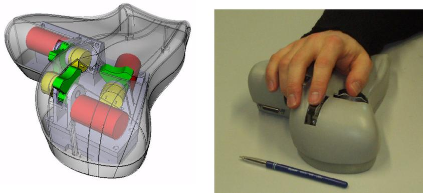
**Fig. 1.** The DigiHaptic with its three levers actuated by motors and the way the user puts his hand on it.
