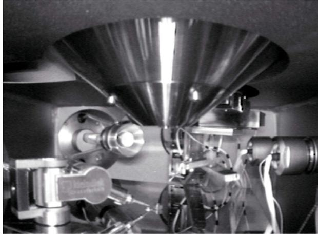
**Fig. 4.** Two microrobots operating in the SEM chamber
