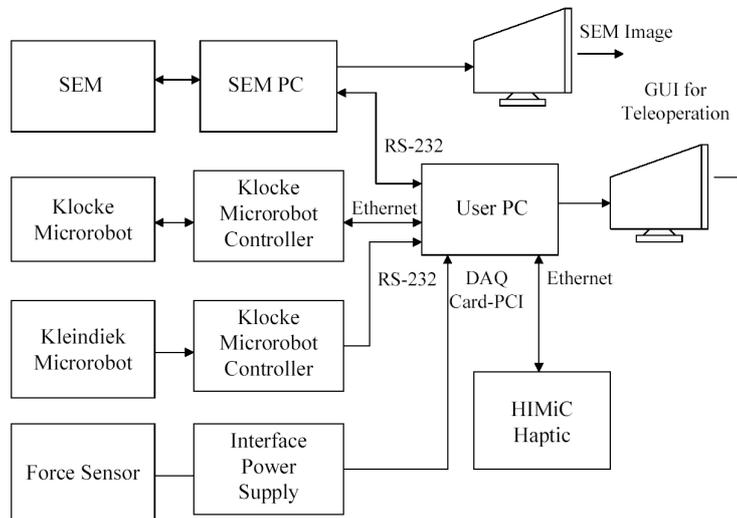
**Fig. 5.** Control structure of the microrobot cell with a haptic interface
