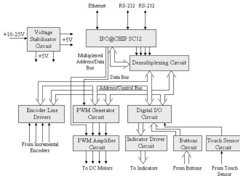
**Fig. 2.** Architecture of electronic circuits of the HIMiC
