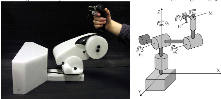
**Fig. 1.** HIMiC haptic device (left) and its kinematic structure (right)
