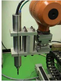
**Fig. 7.** Tool assembly with force sensor
