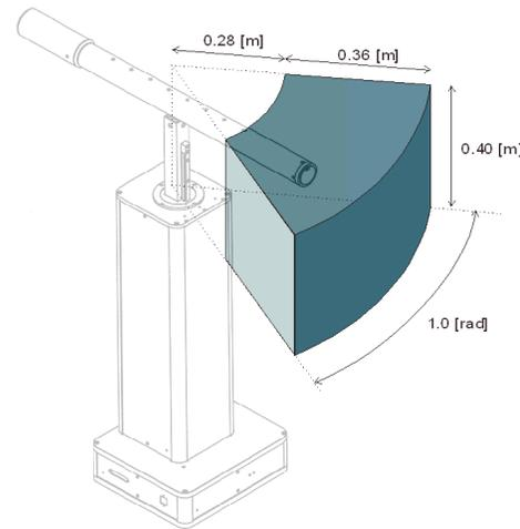
**Fig. 3** The end effector plate workspace of the HapticMaster spans a 3-dimensional space with a volume of approximately 80 liters. The end plate of the robot arm allows the mounting of different end effectors.
