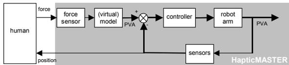
**Fig. 2** The general control scheme of the HapticMaster comprises an outer control loop, and an inner servo loop. A (virtual) model converts the force sensor signal to a Position/Velocity/Acceleration setpoint vector. The inner servo loop controls the robot to the PVA setpoint values.
