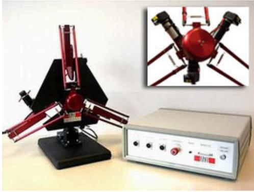
Figure 1: Delta Haptic Device
