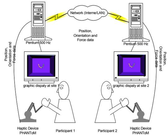
Figure 1. Diagram of the tele-handshake system
